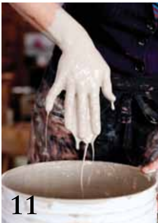
11 Test the consistency of your slip. You want it to web between your fingers.
