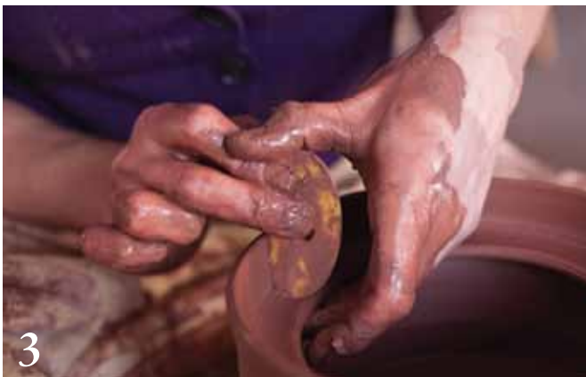
3 Use a small curved rib to put a small indent into the seat to hold the lid.
