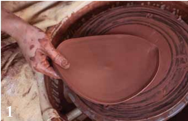
1 Throw a flat disk of clay ¾ to ½-inch thick on the wheel, cut it off of the wheel and stretch into an oblong slab.
