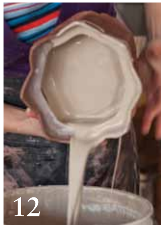
12 Pour white slip into the jar, then rotate it as you pour it out for a thorough coat.
