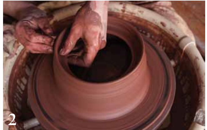
2 Throw a low, thick, open bottomed cylinder. Create a lid seat early in the process and refine it as you pull the wall up.
