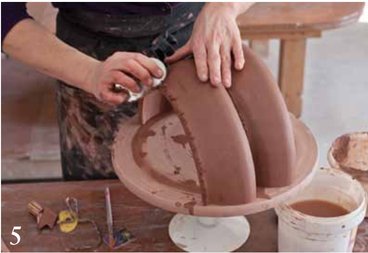
5 Cut the rim into two pieces and score the bottom edge of each one.
