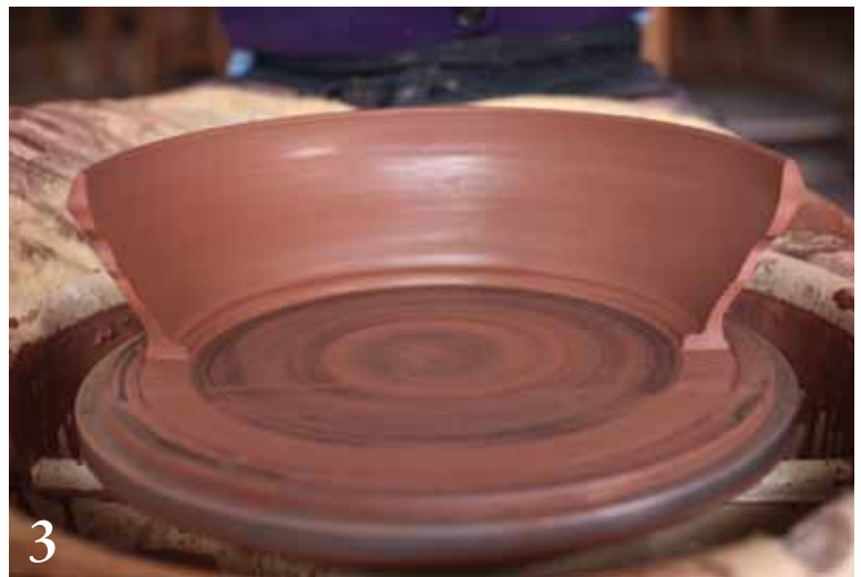
3 Leave a bit of a foot on the rim section to help it stay attached to the wheelhead during throwing
