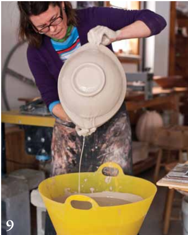
9 Dip the bowl into deflocculated white slip and hold it upside down to let the excess slip run off.
